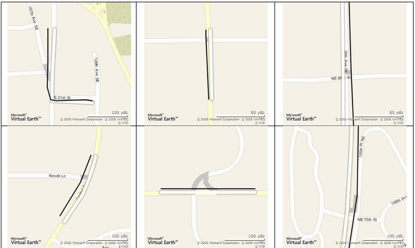
Figure 10: Spur distraction. Our algorithm successfully ignores spurs off the traveled road that distract the nearest road algorithm.
