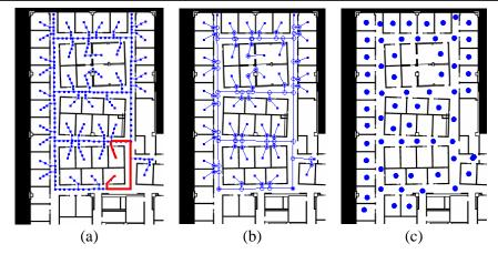
Figure 3: Location Nodes. (a) Dense set of location nodes. The red path shows the shortest path distance between the centers of two offices. (b) Walking paths that were drawn by hand. (c) Sparse set of calibration nodes at which we took signal strength readings.
