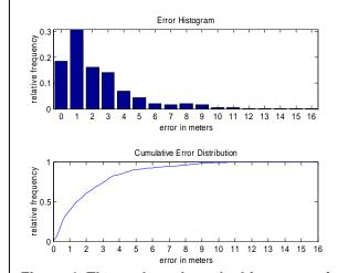
Figure 4: These plots show the histogram of error distances and cumulative error distribution for our test of 4586 different signal strength scans.
