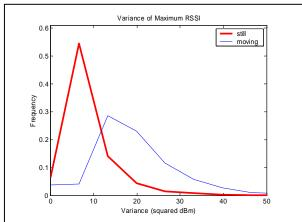
Figure 1: Normalized histograms of the variance of signal strength for a nonmoving and moving device. In general, moving devices show more variance.
