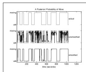
Figure 2: Results from our attempt to infer the probability that a device is moving based on the variance of signal strengths. The middle plot shows the unsmoothed probabilities, which jump around too much compared to the ground truth at the top. The bottom plot shows the probabilities smoothed with an HMM, which come much closer to ground truth.
