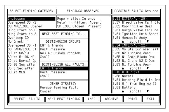
Figure 10: End-user Interface for Turbine Diagnosis.
