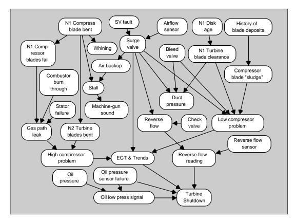
Figure 9: Belief Net for Gas Turbine Diagnosis.
