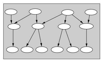
Figure 6: A Singly Connected Belief Network, or Polytree.
